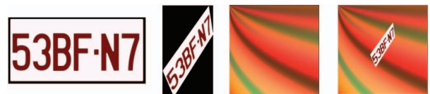
Fig. 2. Adjust the license plate text to the existing style, randomly rotate and scale it and paste it on the randomly generated background.
