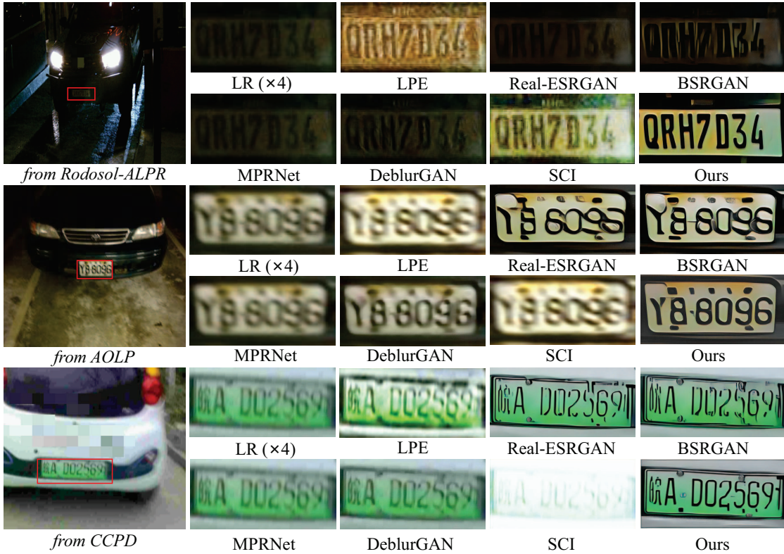
Fig. 4. Qualitative comparisons of different SR methods on real-world LP images with scale factor 4. Better zoom in for details.
