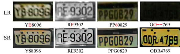
Fig. 5. The sample of correcting the recognition results by the proposed method. Error results are marked in red.
