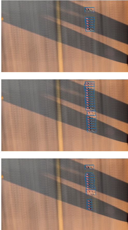
Fig. 5: Stacked detection results across 20 consecutive frames. a) first row: results from the baseline fine-tuned DETR model, b) second row: from seqDETR-3 and c) third row: from seqDETR-5.
