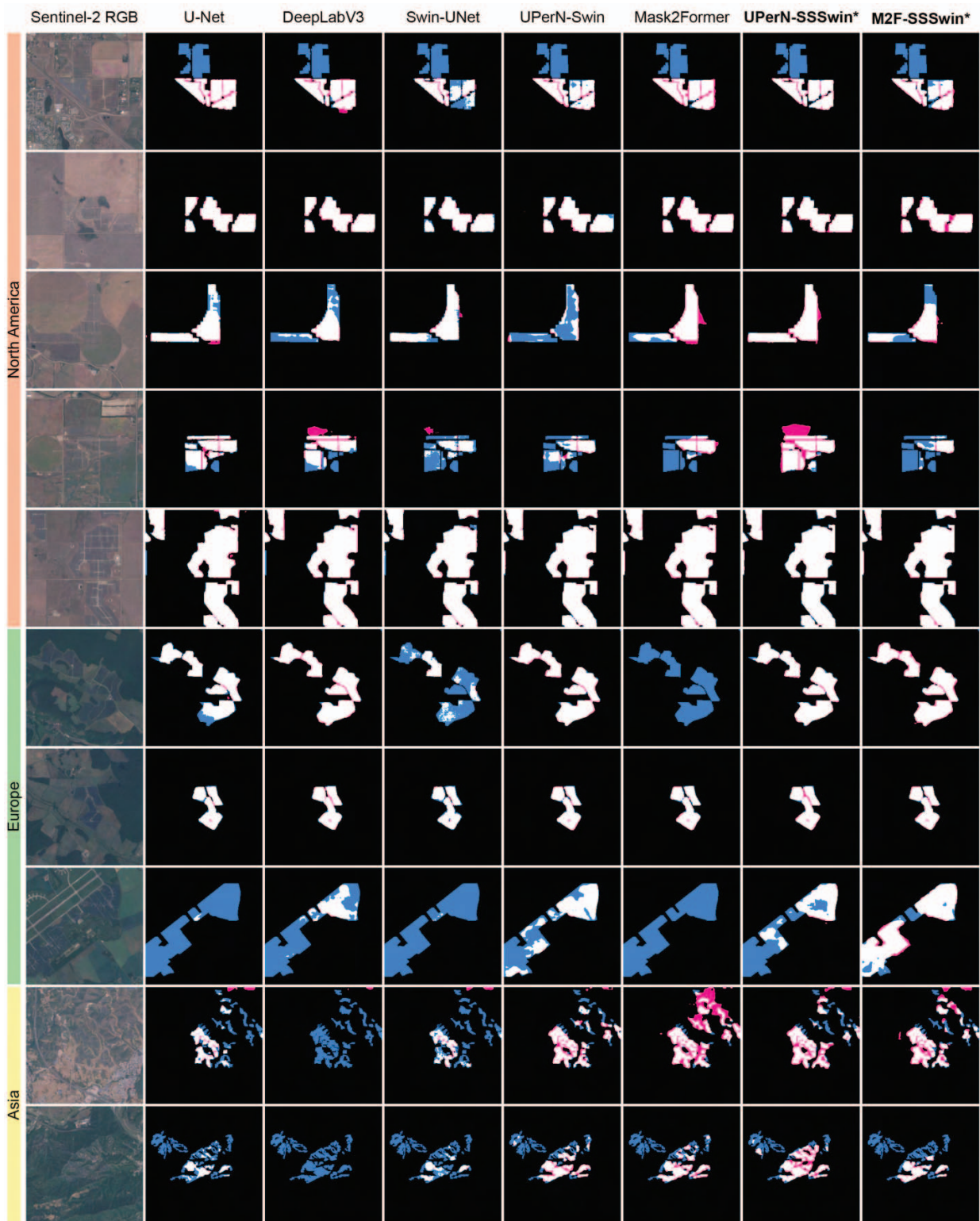
Fig. 6. Qualitative comparison of our predicted solar panel maps (by SSSwin) and the ground truth across different continents. Here, we represent True Positive as white , True Negative as black , False Positive as red , and False Negative as blue .
