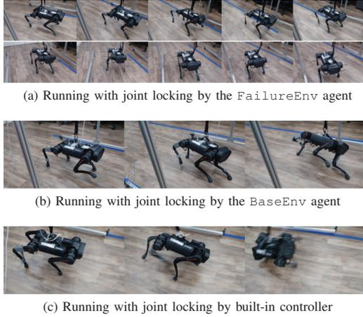
Fig. 4. Deployment snapshots on the physical robot run by (a) fault-tolerant FailureEnv agent with one (top) and two (bottom) joint locked, (b) baseline BaseEnv agent and (c) AI’s built-in controller.
